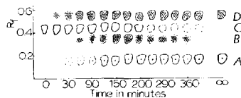
Fig. 3.—Chromatograms illustrating the progress of hydrolysis of 9-methylisoalloxazine in 0.5 N sodium hydroxide and at 45°. Key: A, keto acid; B, anil; C, isoalloxazine; D, dioxo compound.
